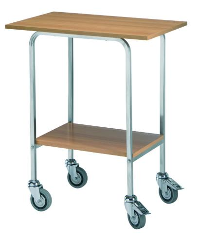
Service trolley gueridon with 2 shelves. Frame in square tube 20x20 mm . Shelves in wood panelled with laminated plastic in walnut colour. 4 swivelling grey rubber castors diam. 100 mm - dim. 700x450x800h mm - 019.L
