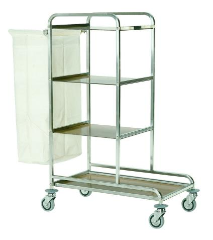
Trolleys for linen, frame made in stainless steel 18/10 AISI 304, square tube 20x20 mm. Shelves made in laminated plastic, bags for linen made in canvas. 4 swivelling wheels Ø 125 mm. 4 bumpers made in PVC, 2 bags made in canvas. Dim. mm 940x480x1320 h - 461.LA
