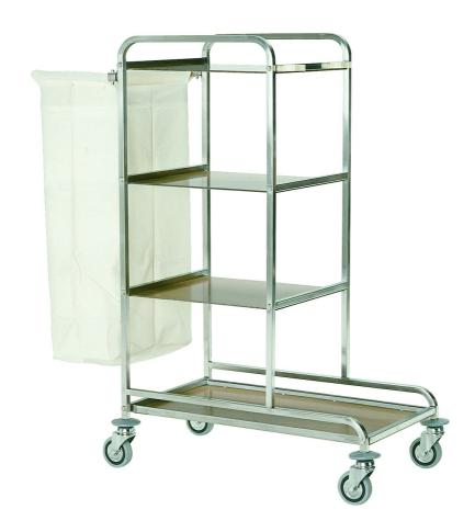
Trolleys for linen, frame made in stainless steel 18/10 AISI 304, square tube 20x20 mm. Shelves made in laminated plastic, bags for linen made in canvas. 4 swivelling wheels  $\emptyset$  125 mm. 4 bumpers made in PVC, 1 bag made in canvas, 1 bag for rubbish made in PVC. Dim. mm 800x400x1040 h - 366.LC
