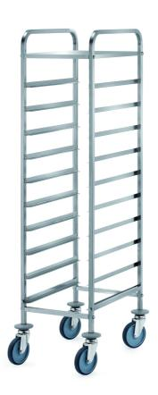
Trolley for trays with upper shelf and railing. Frame made in stainless steel 18/10 AISI 304, square tube 20x20 mm. Upper shelf and railing. 4 swivelling wheels Ø 125 mm, rubber bumpers. Capacity 10 euronorm trays, dim. mm 490x600x1540 h - 634.ES
