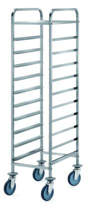
Trolley for trays with upper shelf and railing. Frame made in stainless steel 18/10 AISI 304, square tube 20x20 mm. Upper shelf and railing. 4 swivelling wheels Ø 125 mm, rubber bumpers. Capacity 10 gastronorm trays, dim. mm 450x600x1540 h - 634.AS
