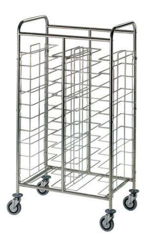
Trolley for trays, universal guides. Frame made in stainless steel 18/10 AISI 304, round tube Ø 25 mm. Guides made in chromium-plate round tube, distance between guides 11 cm. 4 swivelling wheels, rubber bumpers. Capacity 22 trays, dim. mm 900x600x1500 - 611.U/CR
