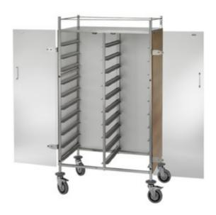
Trolley for trays with lateral with plexiglass panels. Frame made in stainless steel 18/10 AISI 304, square tube 20x20 mm. Covered on 3 sides with thick-antiacid laminated panels, doors made in plexiglass with magnetic closing. Upper shelf and railing. 4 swivelling wheels Ø 125 mm, rubber bumpers. Capacity 20 gastronorm trays, 2 doors. Dim. mm 800x600x1540 h - 638.CH
