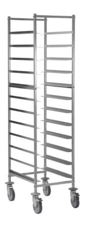
Trolley for trays. Frame made in stainless steel 18/10 AISI 304, square tube 20x20 mm. Guides shaped as "L" depth 50 mm, distance between guides 120 mm. 4 rubber swivelling wheels Ø 125 mm, 4 grey rubber bumpers. Capacity 12 euronorm trays 530x370x115 mm; dim. mm 480x600x1800 - 630.A
