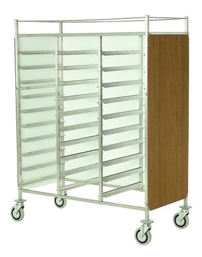
Trolley for trays with upper shelf and railing. Frame made in 18/10 AISI 304 stainless, square tube 20x20 mm. Covered on 3 sides with thick-antiacid laminated panels. Upper shelf and railing. 4 swivelling wheels  $\emptyset$  125mm, rubber bumpers. Capacity 30 euronorm trays, dim. mm 1290x600x1540 h - 639.ES
