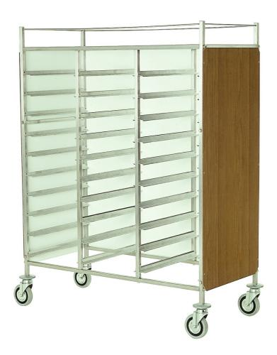
Trolley for trays with upper shelf and railing. Frame made in 18/10 AISI 304 stainless, square tube 20x20 mm. Covered on 3 sides with thick-antiacid laminated panels. Upper shelf and railing. 4 swivelling wheels Ø 125mm, rubber bumpers. Capacity 30 gastronorm trays, dim. mm 1150x600x1540 h -639.AS
