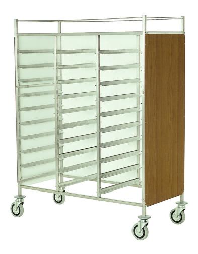
Trolley for trays with upper shelf and railing. Frame made in 18/10 AISI 304 stainless, square tube 20x20 mm. Covered on 3 sides with thick-antiacid laminated panels. Upper shelf and railing. 4 swivelling wheels  $\emptyset$  125mm, rubber bumpers. Capacity 20 euronorm trays, dim. mm 890x600x1540 h - 638.ES
