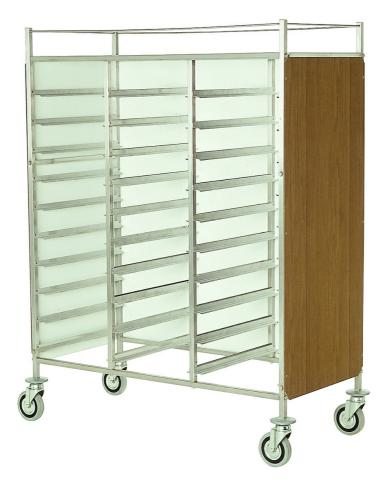
Trolley for trays with upper shelf and railing. Frame made in 18/10 AlSI 304 stainless, square tube 20x20 mm. Covered on 3 sides with thickantiacid laminated panels. Upper shelf and railing. 4 swivelling wheels Ø 125mm, rubber bumpers. Capacity 20 gastronorm trays, dim. mm 800x600x1540 h - 638.AS
