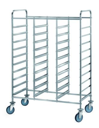
Trolley for trays. Frame made in stainless steel 18/10 AISI 304, square tube 20x20 mm. Runners made in stainless steel 18/10. 4 swivelling wheels Ø 125 mm, rubber bumpers. Capacity 30 gastronorm trays, dim. mm 1150x600x1440 h - 636.A
