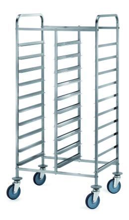
Trolley for trays. Frame made in stainless steel 18/10 AISI 304, square tube 20x20 mm. Runners made in stainless steel 18/10. 4 swivelling wheels Ø 125 mm, rubber bumpers. Capacity 20 euronorm trays, dim. mm 890x600x1440 h - 635.E
