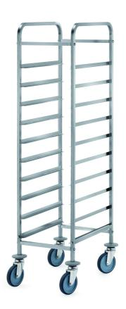
Trolley for trays. Frame made in stainless steel 18/10 AISI 304, square tube 20x20 mm. Runners made in stainless steel 18/10. 4 swivelling wheels Ø 125 mm, rubber bumpers. Capacity 10 euronorm trays, dim. mm 490x600x1440 h - 634.E
