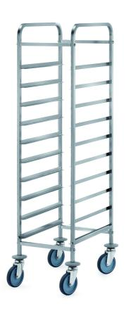
Trolley for trays. Frame made in stainless steel 18/10 AISI 304, square tube 20x20 mm. Runners made in stainless steel 18/10. 4 swivelling wheels Ø 125 mm, rubber bumpers. Capacity 10 gastronorm trays, dim. mm 450x600x1440 h - 634.A
