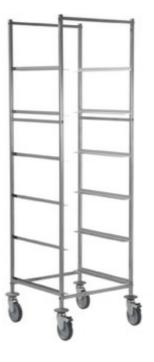
Trolley for dishwasher racks. Frame made in stainless steel 18/10 AISI 304, square tube 25x25 mm, crossbars with bolts. Guides shaped as "L" made in stainless steel, depth 50 mm and thickness 12 mm. 4 wheels Ø 125 mm, 4 grey rubber bumpers. Capacity 6 racks for dishwasher 510x510 mm, distance between guides 250 mm; dim. mm 610x570x1800 h - 633.AS
