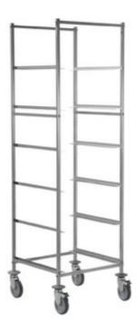
Trolley for dishwasher racks. Frame made in stainless steel 18/10 AISI 304, square tube 25x25 mm, crossbars with bolts. Guides shaped as "L" made in stainless steel, depth 50 mm and thickness 12 mm. 4 wheels Ø 125 mm, 4 grey rubber bumpers. Capacity 10 racks for dishwasher 510x510 mm, distance between guides 300 mm; dim. mm 1150x600x1800 h - 632.A
