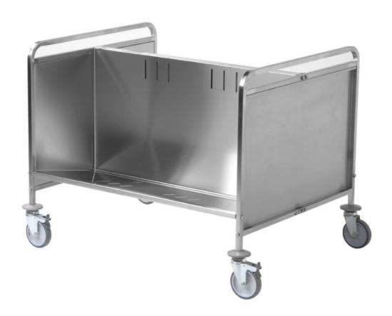
Trolley for plates. Carrying frame in stainless steel AISI 304 18/10, square tube 20x20 mm, reinforced and tilted lower shelf toi carry dishes, cap. 300 kg (400 plates), 4 swivelling castors diam. 125 mm, 2 with brake - dim. 1120x900x850h mm - 343.A
