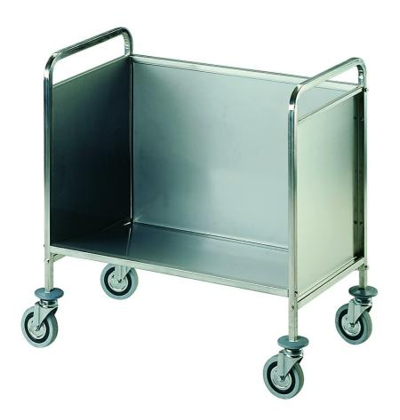
Trolley for plates. Carrying frame in stainless steel AISI 304 18/10, square tube 20x20 mm, reinforced and tilted lower shelf toi carry dishes, cap. 150 kg (200 plates), 4 swivelling castors diam. 125 mm, 2 with brake - dim. 910x570x900h mm - 342.A
