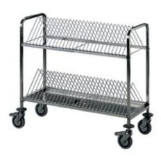
Tray-draining trolley. Carrying frame in stainless steel AISI 304 18/10, draining grids, drop-collecting basin in stainless steel with a plug. 4 swivelling castors diam. 125 mm. Stainless steel grids, cap. 90 trays - dim. 1080x450x1400h mm - 744
