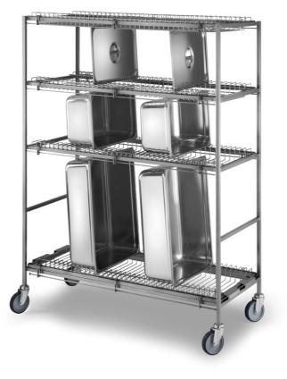
Pots and pans drain trolley GN1/1 and GN2/1. 4 shelves with stainless steel grids, 1 removable shelf. Built-in lock system and anti-overturning system. 4 castors diam. 125 mm - dim. 1250x600x1730h mm -596.A/INOX
