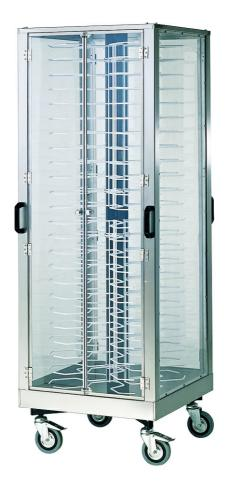
Neutral cabinet trolley for plates. Carrying frame in stainless steel AlSI304 18/10. Cap. 96 plates max diam. 28-32 cm, arranged on 4 rows. Solid base on 4 swivelling castors, 2 with brake; 4 push handles that permit a quicker service and an easy placement in any environment, from the dining room to the refrigerated cell without any problem. Dishholding grids in stainless steel, double opening - dim. 650x650x1860h mm - 346.MA
