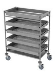
Glass and cup-draining trolley. Carrying frame in stainless steel AISDI 304 18/10, square tuibe 20x20 mm. Stainless steel AISI 304 sliding slotted shelves, drop-collecting basin in stainless steel with plug. 4 swivelling castors diam. 125 mm, 2 with brake. Stainless steel carrying frame, 5 sliding shelves dim. 940x530x1250h mm - 542.A/INOX
