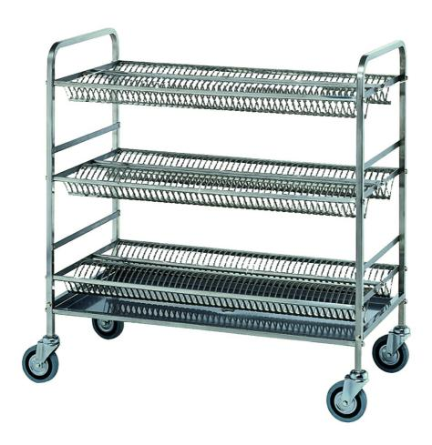
Plate and glass-draining trolley. Carrying frame in stainless steel AISI 304 18/10, square tube 20x20 mm, Grilled shelves in stainless steel, drop-collecting basin in stainless steel with plug. 4 swivelling castors mm 125, 4 plate-draining shelves, cap 360 plates - dim. mm 1060x570x1560h - 347.A/INOX
