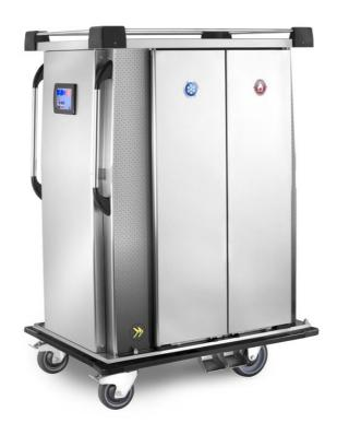
Thermorefrigerated trolley single refrigeration for temperature maintaining with a hot compartment and a cold one for meals packaging line "cold/hot" or "cook and serve". Power 6 Kw. Cap. 24 trays mm 570x325 - dim. 1140x780x1430h mm - MTC24/S
