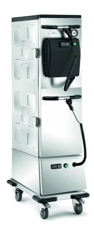
Thermobox trolley mixed version, structure totally made in stainless steel 18/10 AISI 304. With insulated double wall for a good heat retain. Rounded inner corners with deep-drawn slideways for pans, with rounded internal part. Swing door with handle, opening till 180° with rubber gasket, pushing handles on the door. Heated upper part, refrigerated lower part. Temperature control through 2 digital thermostats. 4 wheels diam. 125 mm, 2 of which swivelling with brake
