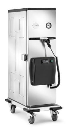
Thermobox trolley heated version with hinged door, 0/+90°C, 900W, 230V, 50/60Hz, cap. 11xGN1/1 H40mm or 5xGN1/1 H100mm + 1xGN1/1 H40mm or 2xGN1/1 H200mm + 3xGN1/1 H40mm. Pitch mm.55. - TNG/11C
