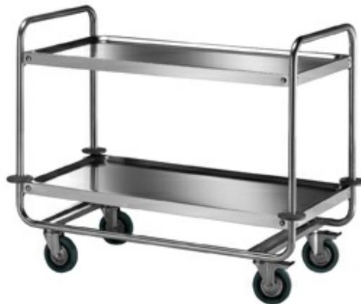
Trolley with pressed shelves, carrying frame made in stainless steel 18/10, round tube  $\varnothing$  25 mm, pressed tray-shaped soundproof shelves made in sating stainless steel 18/10 with perfectly rounded upper and lower edges. 4 grey swivelling rubber wheels  $\varnothing$  125 mm, rubber bumpers. Capacity 130 Kg each shelf. Two-shelves trolley mm 1100x590x900h - 213.A
