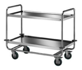
Shelves trolley made in 18/10 stailess steel, carrying frame made in 18/10 stainless steel, round tube Ø 25 mm, tray-shaped soundproof shelves made in sating 18/10 stainless steel with perfectly rounded upper and lower edges. 4 grey rubber swivelling wheels Ø 125 mm, rubber bumpers. Two-shelves trolley mm 1280x680x900h - 211.AG
