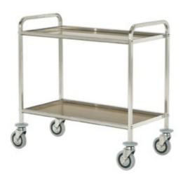
Trolley with laminated shelves, carrying frame made in stainless steel 18/10, square tube 20x20 mm, shelves made in antiacid laminated plastic, walnut colour. 4 grey rubber swivelling wheels Ø 125 mm, rubber bumpers. Two-shelves trolley mm 950x510x900h - 214.LA
