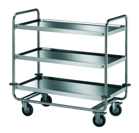
Shelves trolley made in 18/10 stailess steel, carrying frame made in 18/10 stainless steel, round tube Ø 25 mm, tray-shaped soundproof shelves made in sating 18/10 stainless steel with perfectly rounded upper and lower edges. 4 grey rubber swivelling wheels Ø 125 mm, rubber bumpers. Two-shelves trolley mm 1280x680x1020h - 313.AG
