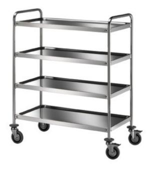
Shelves trolley made in 18/10 stainless steel, carrying frame made in 18/10 stainless steel, round tube Ø 25 mm, tray-shaped soundproof shelves made in sating 18/10 stainless steel with perfectly rounded upper and lower edges. 4 grey rubber swivelling wheels Ø 125 mm, rubber bumpers. Four-shelves trolley mm 1100x680x1250h - 414.AB
