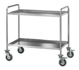
Shelves trolley made in 18/10 stainless steel, welded frame made in stainless steel, round tube Ø 25 mm, knit structure, bended shelves h 30 mm. 4 grey rubber swivelling wheels Ø 125 mm, rubber bumpers. Two-shelves trolley mm 1020x600x900h - 219.A
