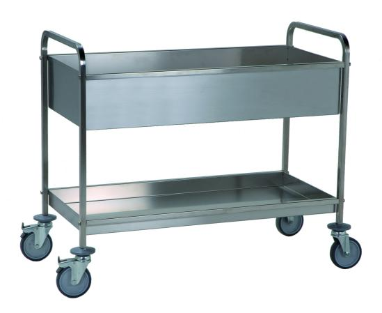
Trolley for differentiated collection, carrying frame made in stainless steel 18/10, square tube 20x20 mm, lower shelf mm 60h. 4 grey rubber swivelling wheels Ø 125 mm, rubber bumpers. Three-shelves trolley mm 1160x560x1020h - 402.AB
