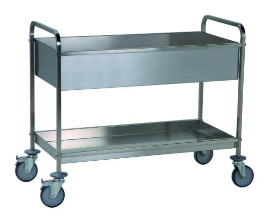
Trolley for differentiated collection, carrying frame made in stainless steel 18/10, square tube 20x20 mm, removable bended shelves mm 60h. 4 grey rubber swivelling wheels Ø 125 mm, rubber bumpers. Three-shelves trolley mm 1100x560x1020h. - 402.A
