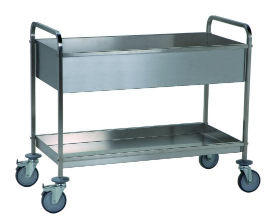
Trolley for differentiated collection, carrying frame made in stainless steel 18/10, square tube 20x20 mm, lower shelf mm 60h. 4 grey rubber swivelling wheels Ø 125 mm, rubber bumpers. Two-shelves trolley mm 1160x560x900h - 401.AB
