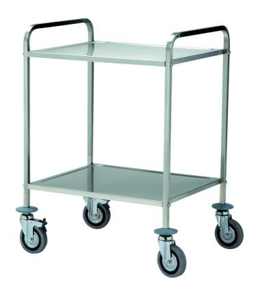
Shelves trolley made in 18/10 stainless steel, carrying frame made in 18/10 stainless steel, square tube 20x20 mm bended shelves h 20 mm, 4 grey rubber swivelling wheels 125 mm, rubber bumpers. Two-shelves trolley mm 700x560x1020h - 204.AC
