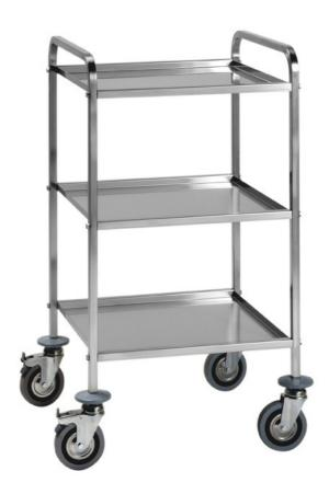
Shelves trolley made in 18/10 stainless steel, carrying frame made in 18/10 stainless steel, square tube 20x20 mm bended shelves h 20 mm, 4 grey rubber swivelling wheels 125 mm, rubber bumpers. Three-shelves trolley mm 800x560x1020h - 302.AC
