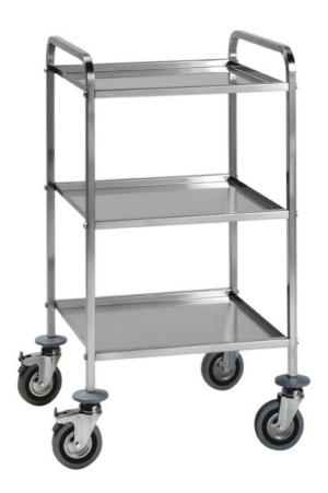
Shelves trolley made in 18/10 stainless steel, carrying frame made in 18/10 stainless steel, square tube 20x20 mm bended shelves h 20 mm, 4 grey rubber swivelling wheels 125 mm, rubber bumpers. Three-shelves trolley mm 800x560x900h - 301.AC
