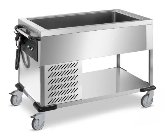
Refrigerated trolley (GN not included). Carrying frame made in stainless steel 304 AISI 18/10. Pressed no-drops basin h 200 mm. Temperature controlled by a digital thermostat; refrigerating system, consisting of HP 1/8 500 W - 230 V 50/60Hz. Spiral cable with CE plug and socket hoot. Push handle. 4 grey rubber swivelling wheels Ø 125 mm not marking, 4 bumpers made in black PVC. Refrigerated trolley, capacity 2 GN1/1 h 200 mm, mm 850x640x900 h - 0131.AB
