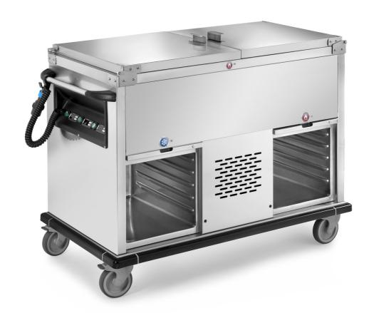
Heated bain-marie trolley separated basins with tilting lids, structure completely made in stainless steel 18/10 AISI 304. Dry/bainmarie heating, temperature controlled by digital thermostat 30° - 90° C° 230 V 50/60 Hz. Insulated lids are opening up to 180°. Deep-drawn separated basins with rounded corners, for 3 GN1/1 H 200, anti-drop board, insulated double wall, spiral electrical wire with CE plug and hooker for the plug, ergonomic push handle, Under compartments with
