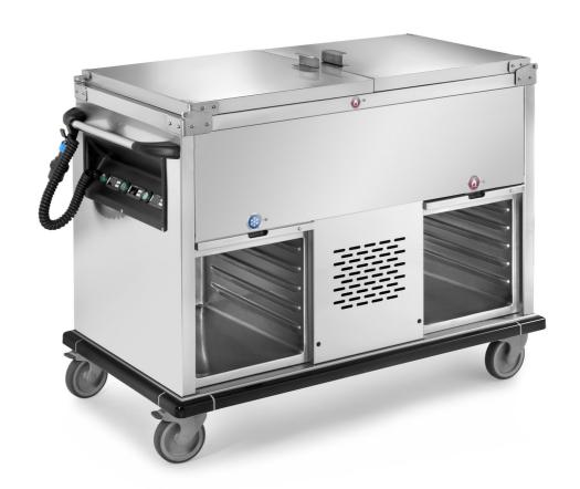
Heated bain-marie trolley separated basins with tilting lids, structure completely made in stainless steel 18/10 AISI 304. Dry/bainmarie heating, temperature controlled by digital thermostat 30° - 90° C° 230 V 50/60 Hz. Insulated lids are opening up to 180°. Deep-drawn separated basins with rounded corners, for 2 GN1/1 H 200, anti-drop board, insulated double wall, spiral electrical wire with CE plug and hooker for the plug, ergonomic push handle, Under compartments with
