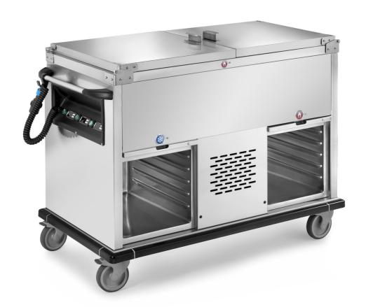
Heated bain-marie trolley unique basin with tilting lids, structure completely made in stainless steel 18/10 AISI 304, dry/bainmarie heating, temperature controlled by digital thermostat 30° - 90° C°. Insulated lids are opening up to 180°. Printed unique basin with rounded corners, for 3 GN1/1 h 200, anti-drop board, insulated double wall, spiral electrical wire with CE plug and hooker for the plug, ergonomic push handle. Under compartments with hiding tilting doors, with 5 printed
