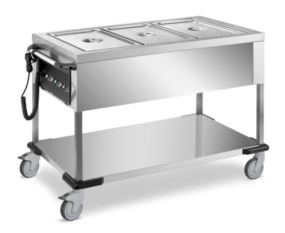
Heated trolley with separated basins (GN not included). Welded frame made in stainless steel 18/10 AISI 304. Pressed no-drops basin divided in sections 1/1 GN, double isolated wall. Temperature of each compartment controlled by a mechanical thermostat 30° - 90° C°. Heating by electrical contact resistance out side the basin 230 V 50/60 Hz. Spiral cable with CE plug and socket hook; push handle. 4 grey not making, rubber swivelling wheels Ø 125 mm, 2 with brake, 4 bumpers
