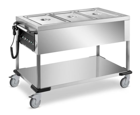
Heated trolley with separated basins (GN not included). Welded frame made in stainless steel 18/10 AISI 304. Pressed no-drops basin divided in sections 1/1 GN, double isolated wall. Temperature of each compartment controlled by a digital thermostat 30° – 90° C°. Heating by electrical contact resistance out side the basin 230 V 50/60 Hz. Spiral cable with CE plug and socket hook; push handle. 4 grey not making, rubber swivelling wheels Ø 125 mm, 2 with brake, 4 bumpers
