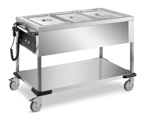
Heated trolley with pressed no-drops basin bain-marie and dry heating (GN not included). Welded frame made in stainless steel 18/10 AISI 304, square tube 30x30 mm. Pressed no-drops basin for GN h 200 mm, double and insulated wall. Temperature controlled by a digital thermostat 30°-90° C°. Spiral cable with CE plug and socket hook; push handle. Heating by electrical contact resistance functioning bain-marie and dry ways 230 V 50/60 Hz. 4 grey not marking rubber swivelling
