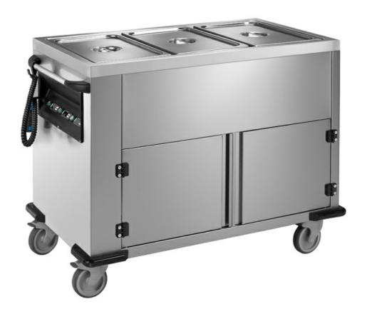
Cabinet heated trolley with separated basins (GN not included), structure completely made in stainless steel 18/10 AISI 304. Pressed nodrops basin divided in sections 1/1 GN H 200, double insulated wall and anti-drop board. Lower compartment closed by swing doors. Temperature of each compartment controlled by a digital thermostat 30° - 90° C°. Heating by electrical contact resistance 500W dry/bainmarie functioning 230 V 50/60 Hz. Cable spiral-shaped with CE
