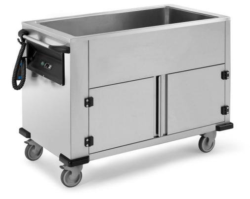
Heated trolley with unique deep-drawn basin (GN not included). Frame made in stainless steel 18/10 AISI 304. Deep-drawn basin for GN h 200 mm with rounded angles, double and insulated wall, neutral lower compartment closed by swing doors. Temperature controlled by digital thermostat 30° - 90° C°. Spiral cable with CE plug and socket hooks; push handle. Heating by electrical resistance external to the basin functioning bain-marie and dry ways 230 V 50/60 Hz. 2 grey not
