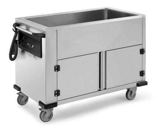
Heated trolley with unique deep-drawn basin (GN not included). Frame made in stainless steel 18/10 AISI 304. Deep-drawn basin for GN h 200 mm with rounded angles, double and insulated wall, neutral lower compartment closed by swing doors. Temperature controlled by digital thermostat 30° - 90° C°. Spiral cable with CE plug and socket hooks; push handle. Heating by electrical resistance external to the basin functioning bain-marie and dry ways 230 V 50/60 Hz. 2 grey not
